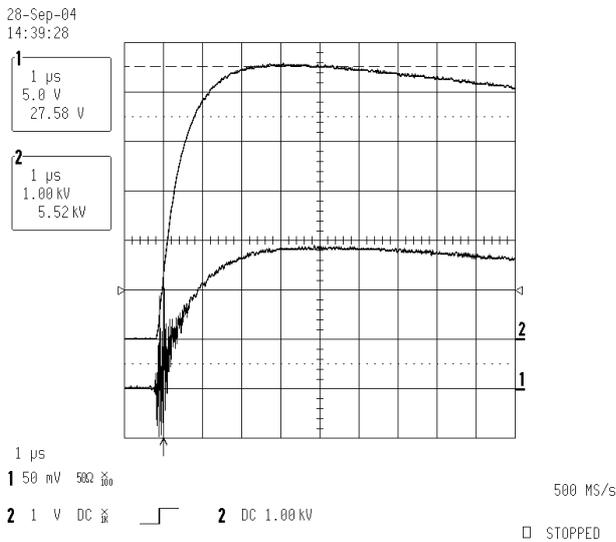
Figure 5 – Voltage and current waveforms from a test on GEM using a 3kA, 8/20  $\mu$ s surge current.
