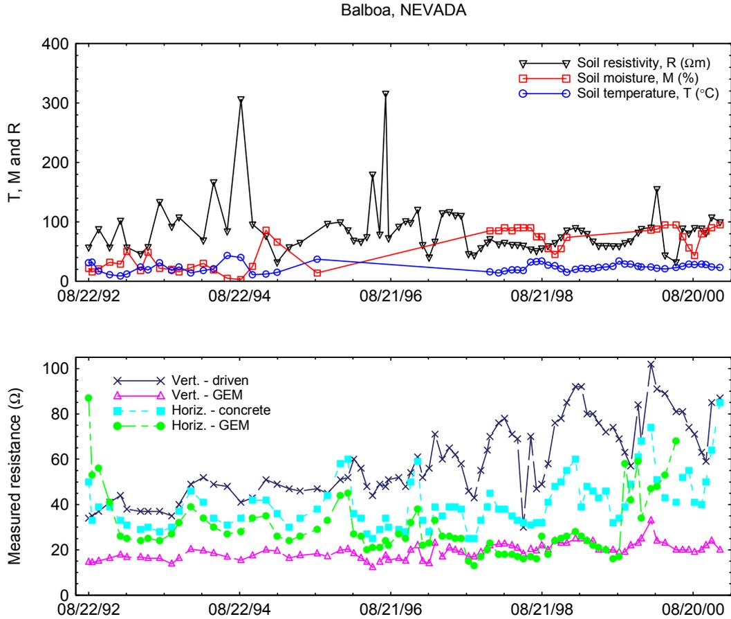
Figure 1 – More than 8 years of grounding resistance data for the Balboa site in Nevada, USA.
