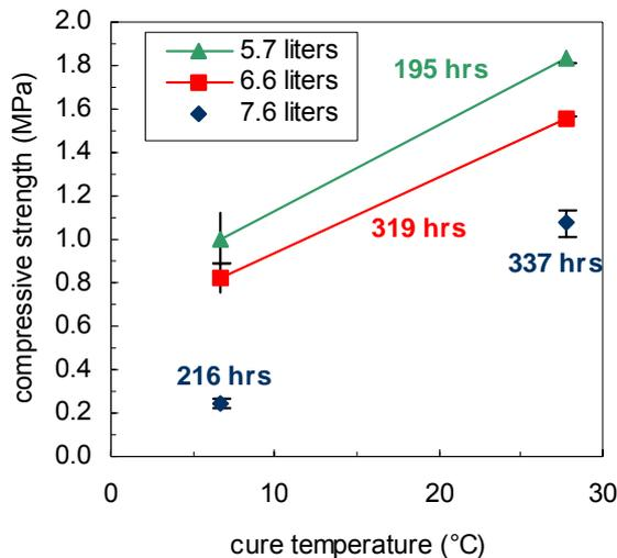
Figure 3 – The effect of temperature on compressive strength of GEM at different mix ratios and curing times. The cure time is indicated for separate data points (7.6 liter) or for all points associated with a linear regression (5.7, 6.6 liters).
