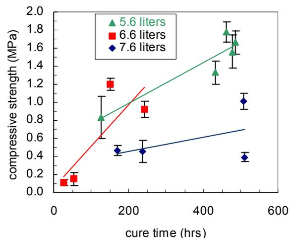
Figure 2 – Compressive strength of GEM for a range of curing times (27 – 511 hrs) and mix ratios (5.7, 6.6, 7.6 liters).
