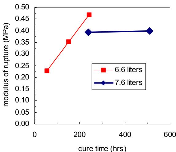
Figure 4 – The effect of cure time on the flexural strength at different mix ratios (6.6, 7.6 liters).
